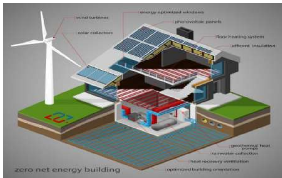
Figure 1: Integrated NetZero Energy Featured Building
